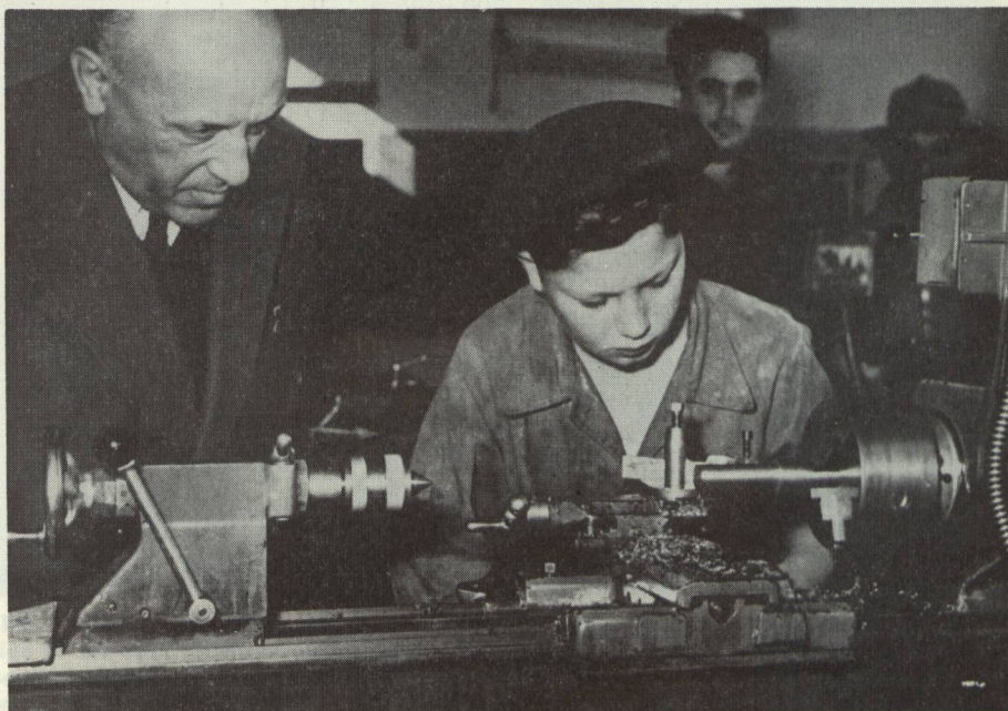
Israel's Minister of Labor, M. Namir, looks on as a youngster in the Machinists School at the Givatayim ORT Center turns a metal rod on a lathe.
